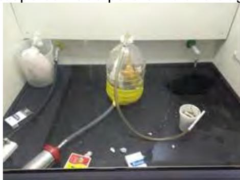
**Figura 2:** Protótipo utilizado para simular a tragada do narguilé
