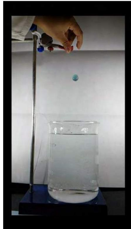
With that, the program initialized the “tracking phase”; in this step, we selected the frame that indicated the beginning of the marble’s movement. From this frame on, we selected in each frame the mass center of the marble, until the mass reached the bottom of the beaker. It was noted that the precision in this step was essential to plot accurate graphics.
